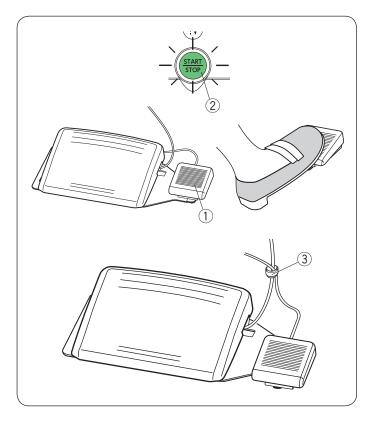
After sewing, depress the thread cutter switch ① on the right side of the foot control to trim the both needle and bobbin threads.
