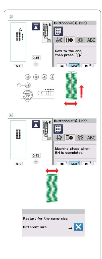
3 Start sewing again, and the machine sews the front bartack and right side of the buttonhole. Stop the machine when you reach the ending point. Then press the reverse button ①.
