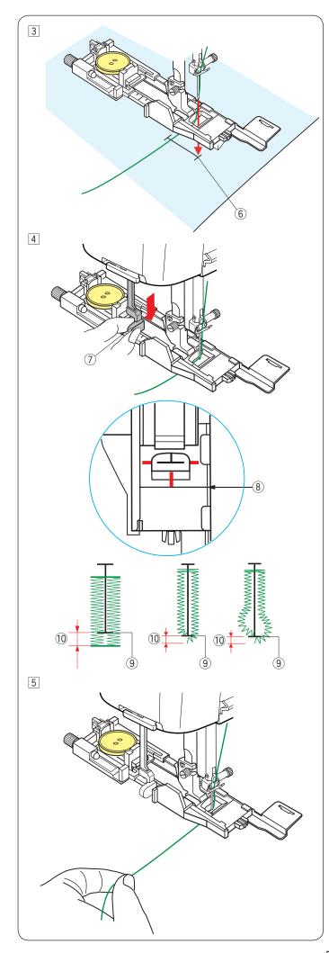
3 Draw the needle thread to the left through the hole of the foot.
